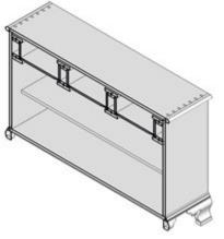
section in the vertical front plane, but sections can be made in any plane, including complex sections by simply rotating the sectioning plane in one or two axes. Sections can be saved as a view and can be dimensioned just like any other view.
